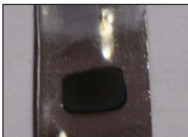
Fig. 4. Oxidized tantalum foil with photodeposited PPy. The polymer layer grows just in that part of the electrode interacting with photons.
